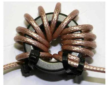
**IMPORTANT** : this **#31 type ferrite** is especially developed for use in common mode chokes, and will give the best wide band results.
