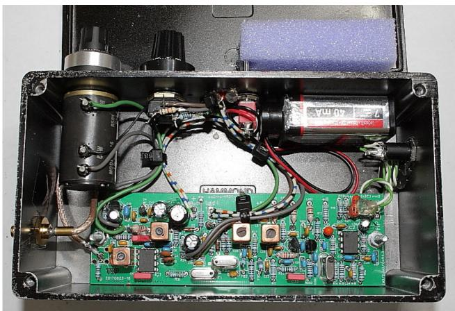
After assembling, and checking all voltages, adjust the receiver for maximal sensitivity using a professional RF signal generator.
