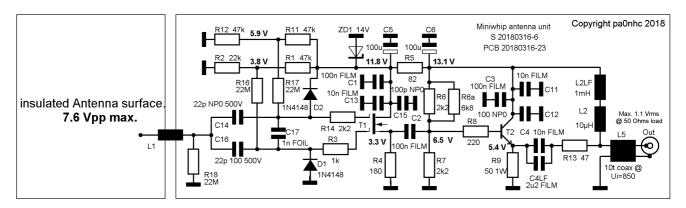
Here the full schematic diagram of the by PA0NHC improved miniwhip antenna unit. The left part shows my unique development. During maximal level signal level drive from the antenna surface, it ensures a constant optimal voltage difference between gate1 and gate2. When the bias voltage difference between gate1 and gate2 of the FET is constant (does not vary), the steepnes of the FET is also constant. Resulting in NO distortion and optimal high signal level properties.
