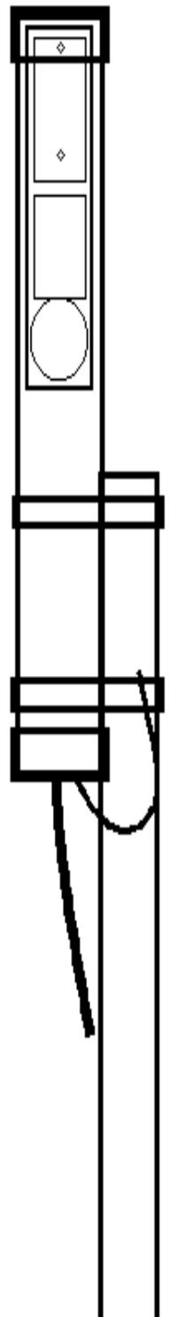
Pa0nhc improved version of Pa0rdt "Miniwhip" active wideband receiving antenna.
