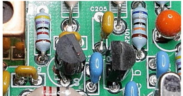
Correct position of adapted BF256b (left) in PCB 20140909-15
