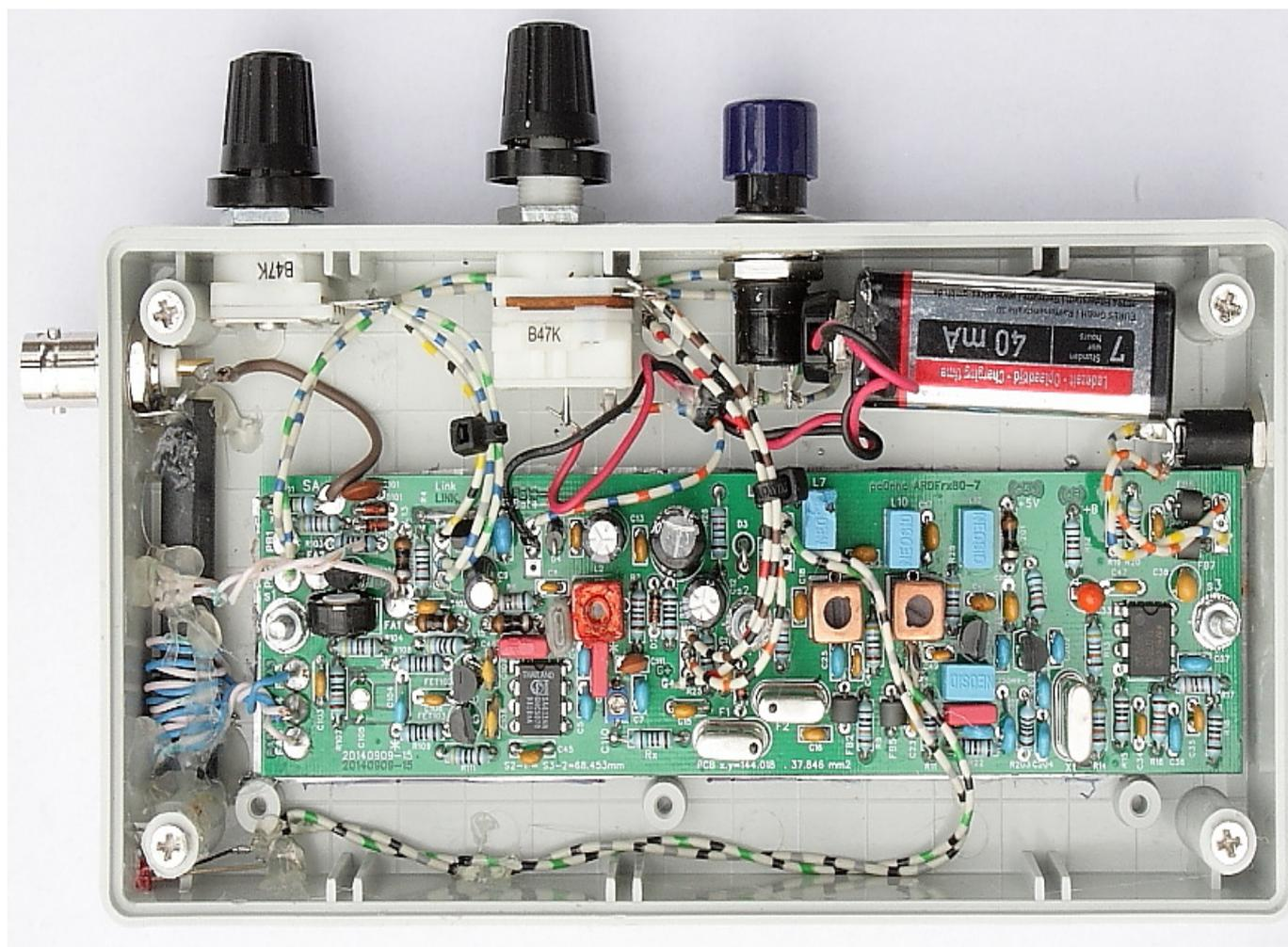
10. Connect all external components (Sa, Pb, Fa, Tune, Gain, Bat, Phone) with supple wires. REM: keep all wires away from the oscillator circuit environment, as a little movement could detune the receiver. After testing, fix the wires with some glue to hold them steady in place.
