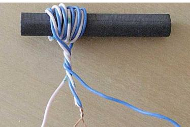
6. Lay the ferrite antenna inside the box in the corner where it later on will be fixed.
