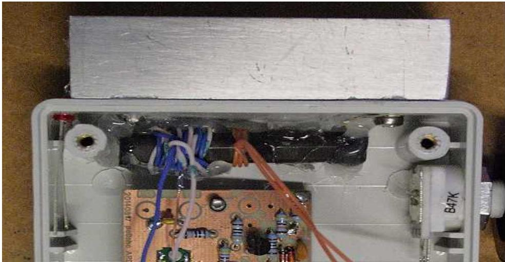
The above shown small ferrite rod (Conrad 535575) nicely fits inside a small 8.5cm x 17cm x 3cm Hammond 1599 ABS box. A 50x20x20mm piece of square ALU pipe could function as **sense antenna**, screwed on top of the box.
